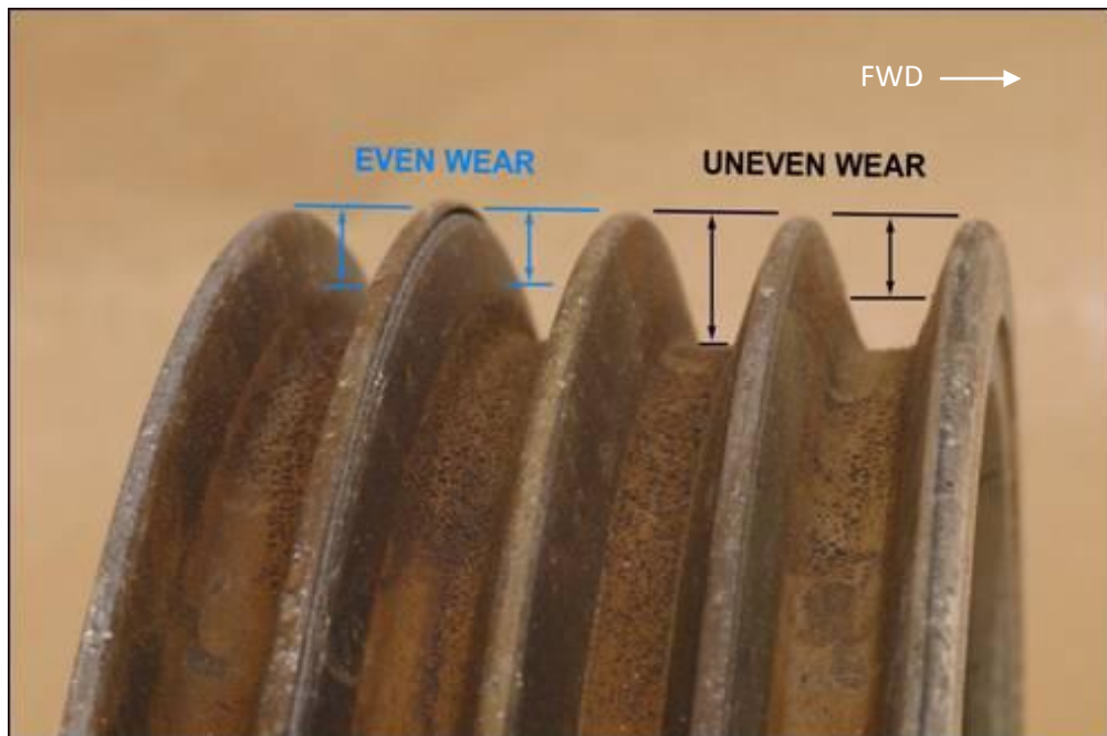
Figure 8: Upper sheave wear pattern
