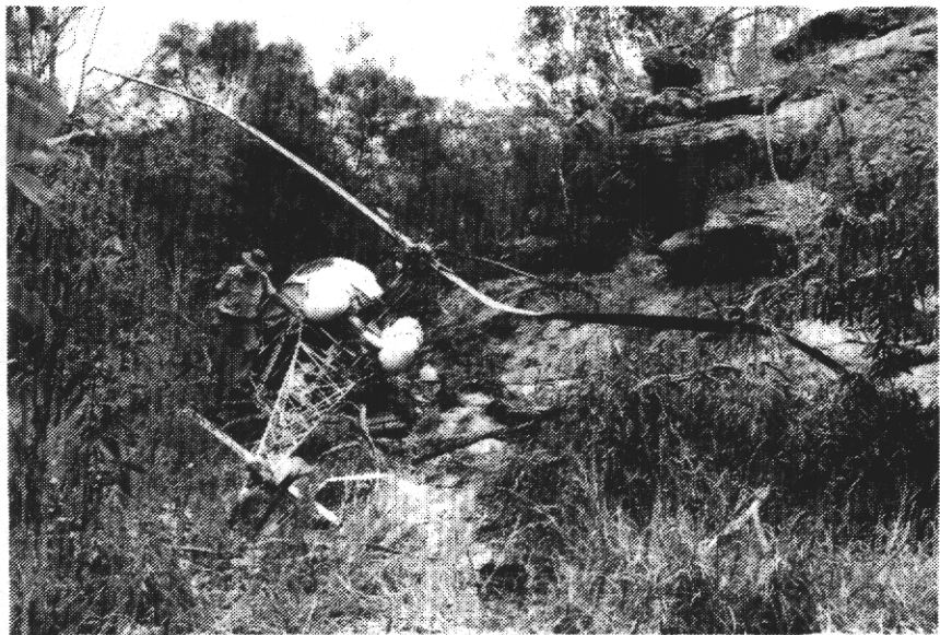
Bell 47- survey flight , overpitched in high density altitude
