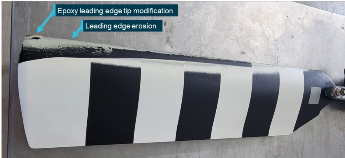
Figure 3: Tail rotor blade leading edge erosion and blade modification
