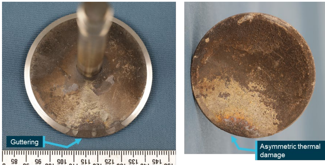
Figure 4: Damaged engine intake valve from number-four cylinder
