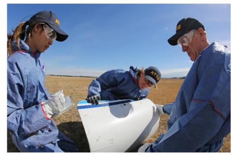
ATSB investigators examine an engine cowling from an aircraft.
