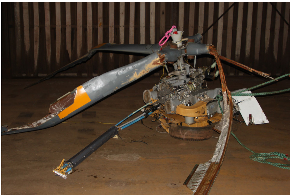
Figure 17: Main rotor blades and main transmission, showing damage in vicinity of the blade roots
