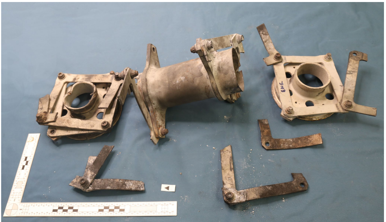
Fragmented KAflex from the accident helicopter, source ATSB
