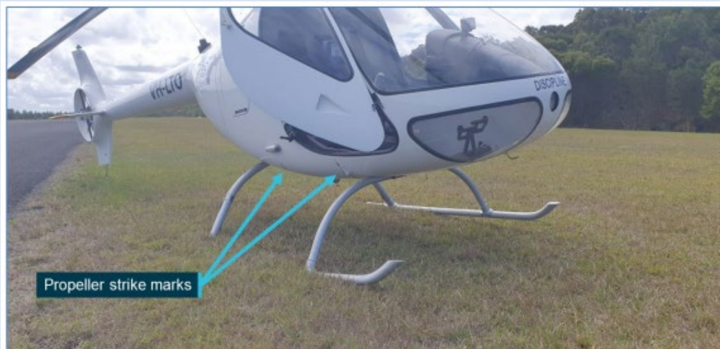
Propeller strike mark and skid damage to VH-LTO
