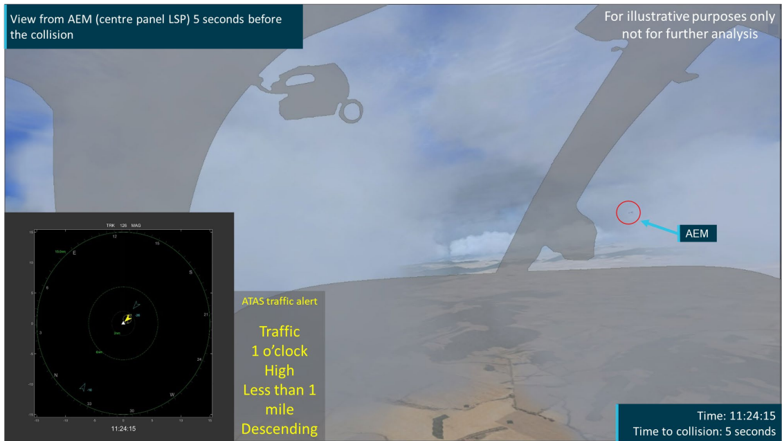
Figure 147: View from JQF LSP 5 seconds before the collision
