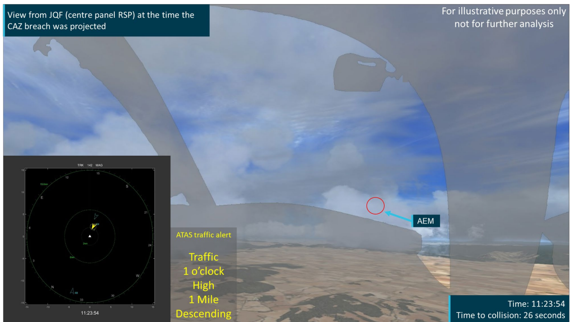
Figure 142: View from JQF RSP when AEM triggered CAZ breach and ATAS alert
