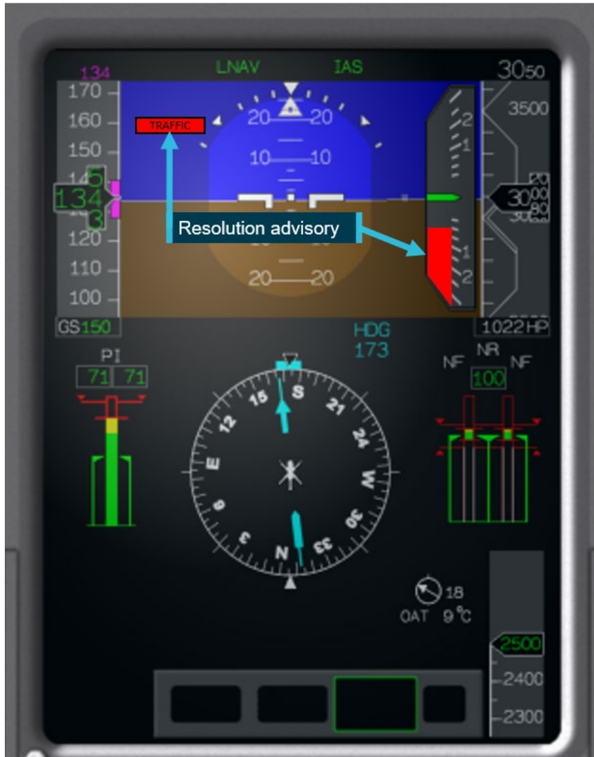
Figure 5: Example of a TCAS 'monitor vertical speed' RA
