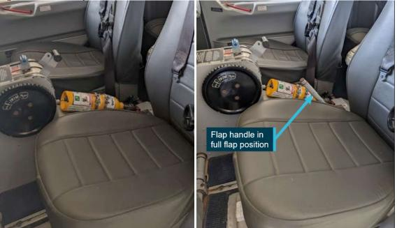
Note: The flap lever rests below the pilot seat bolster and is not visible in the retracted and first stage positions (left). The flap lever protrudes above the bolster in the full flap position (right).
