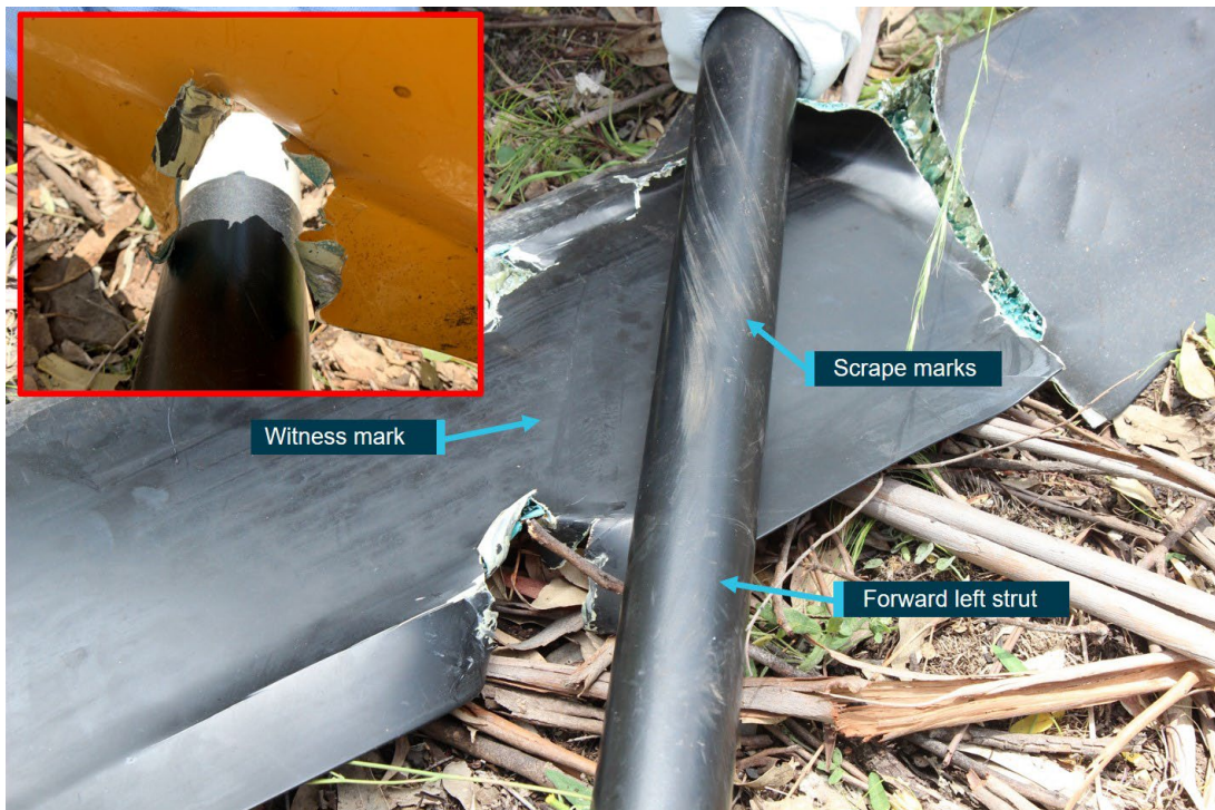
Figure 7: Damage to the blue main rotor blade and the forward left landing strut
