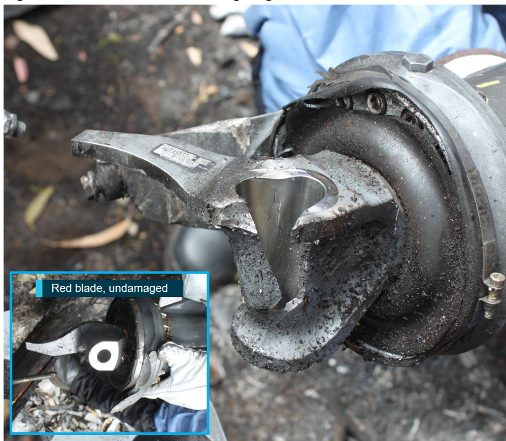
Figure 5: Blue blade tusk and coning hinge bolt bore
