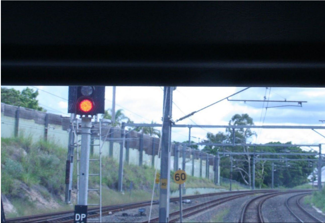
Figure 6: A view of signal DP29 from the driver's seat of an NGR service stopped at the 6-car stopping mark at platform 2 Park Road
