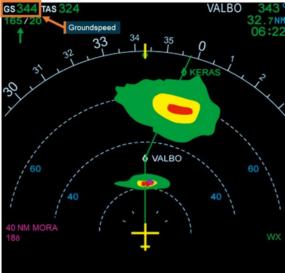
The ND has a number of selectable display modes, including weather radar as shown.
