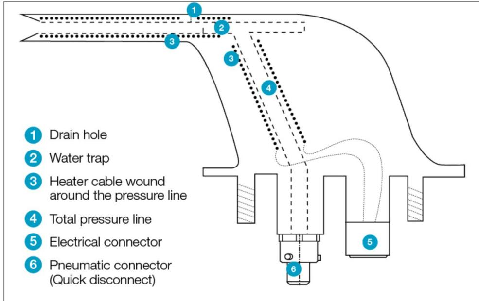
*Representative only; the drawing shows a Thales pitot probe and not a UTC Aerospace Systems pitot probe as used on 9M-MTK.*
