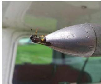
**Figure 3.** Mud Dauber wasp emerging from an uncovered pitot tube.
