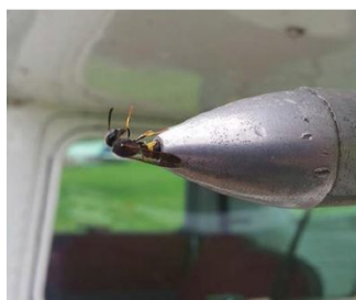
Figure 3. Mud Dauber wasp emerging from an uncovered pitot tube.
