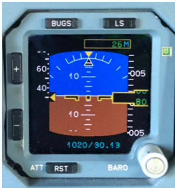
Figure 21: ISIS showing airspeed (left) at the bottom of the scale (30 kt)
