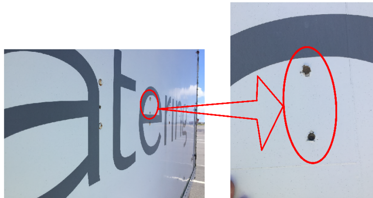
Figure 11. Wasp nest in catering truck panel holes
