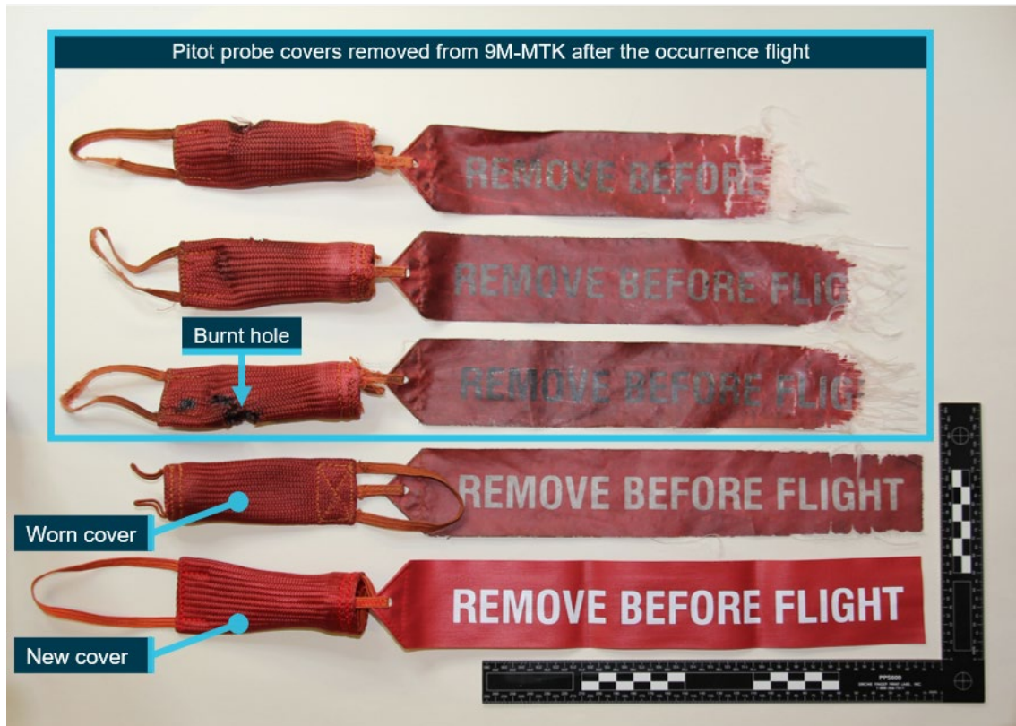
Figure 34: Pitot probe covers removed from 9M-MTK after the occurrence flight, and exemplar covers of the same type
