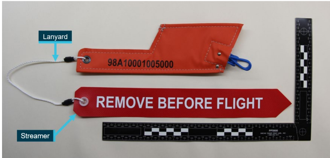
Figure 35: Airbus-approved pitot probe cover with lanyard and streamer
