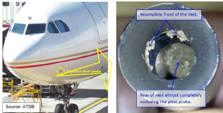
Figure 7. Airbus A330 Wasp Nest Partial Blockage of Captain's Pitot Probe
