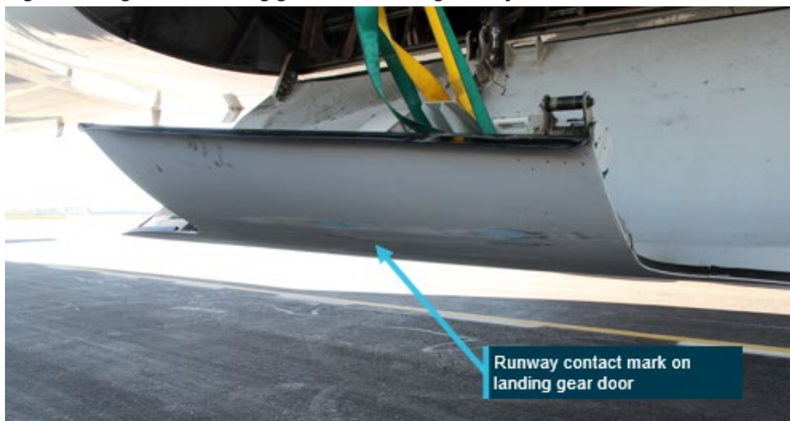
Figure 10: Right main landing gear door showing runway contact mark
