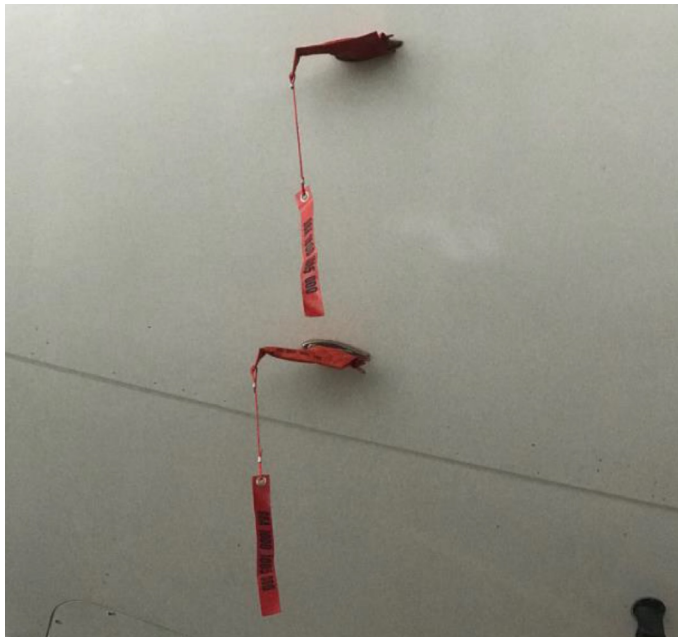
Figure 36: Airbus-approved pitot probe covers fitted to the left side pitot probes of an A330
