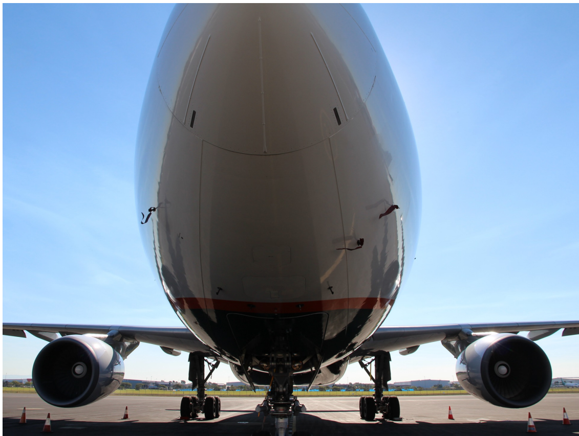
Figure 16: View of an exemplar A330 from eye level, with similar pitot probe covers to those used on the occurrence aircraft
