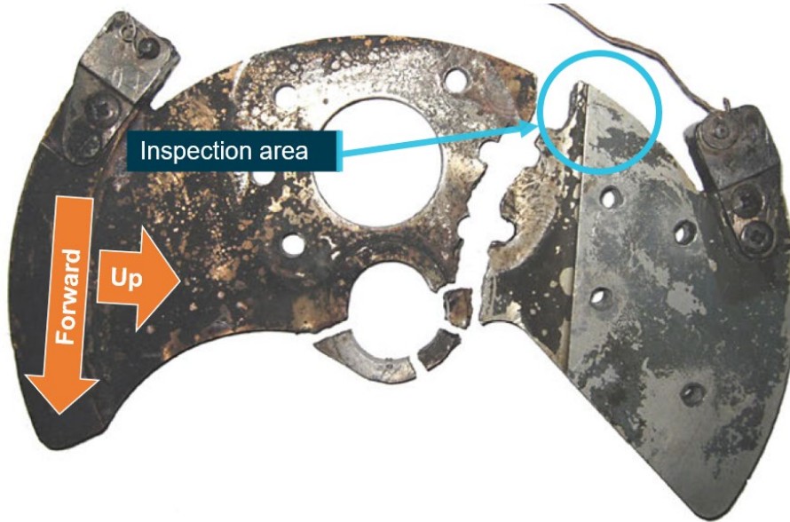
Figure 8: Yak-52 elevator bellcrank from the 2010 Yekaterinburg accident
