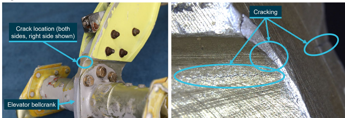
Figure 6: Elevator bellcrank cracks observed on VH-PAE
