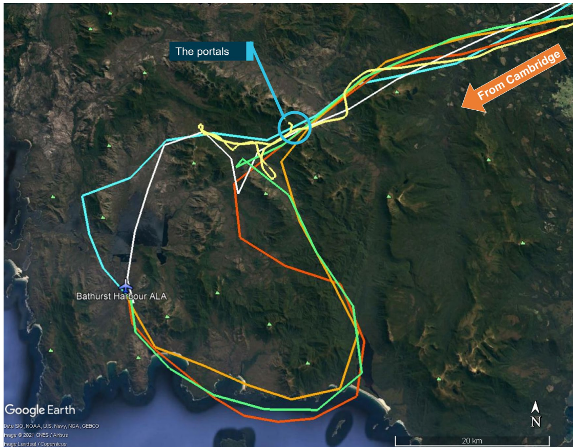
Figure 12: Comparison of aircraft tracks through the valley, including about 1 month prior to the accident (green – lead aircraft; orange – second aircraft) and the accident track (pale yellow)
