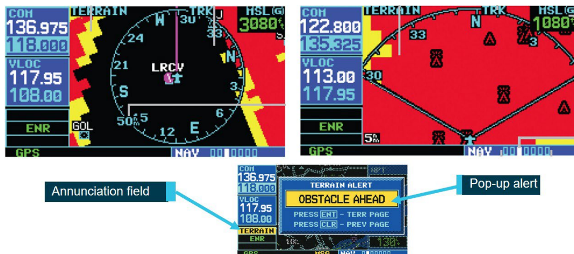
Figure 3: GNS430 alert functions in 360° (left) and 120° (right) views above; alert types below
