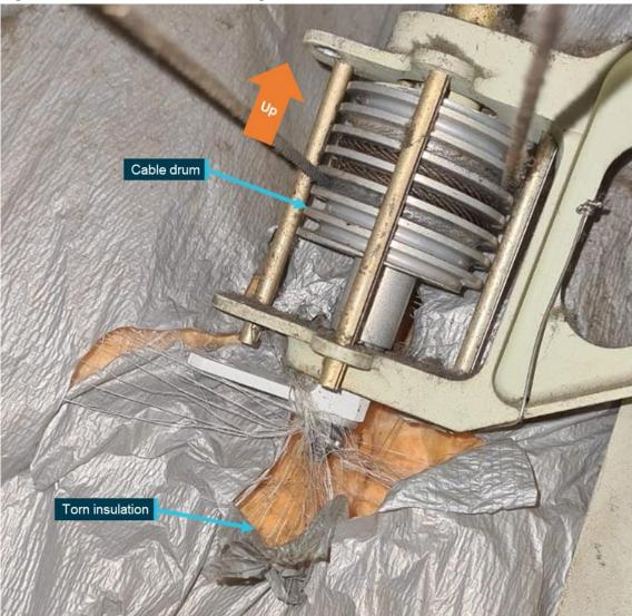
Figure 5: Torn insulation surrounding cable drum
