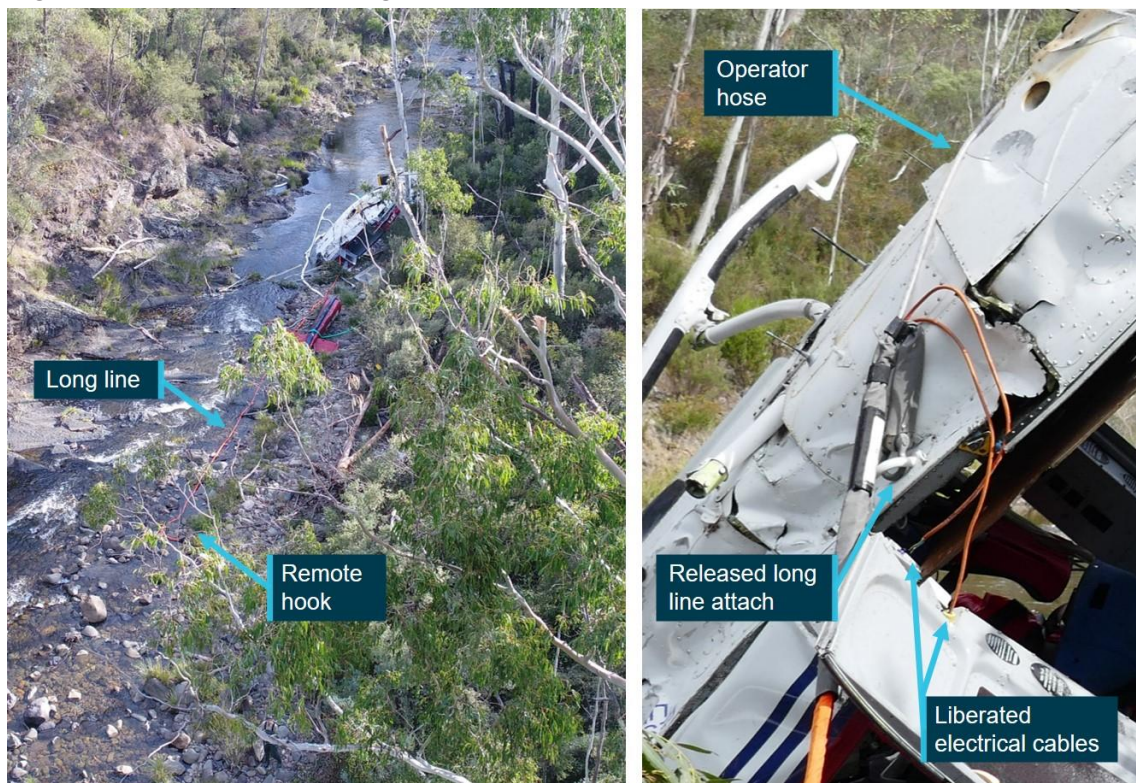
Figure 6: Failed to detach long line
