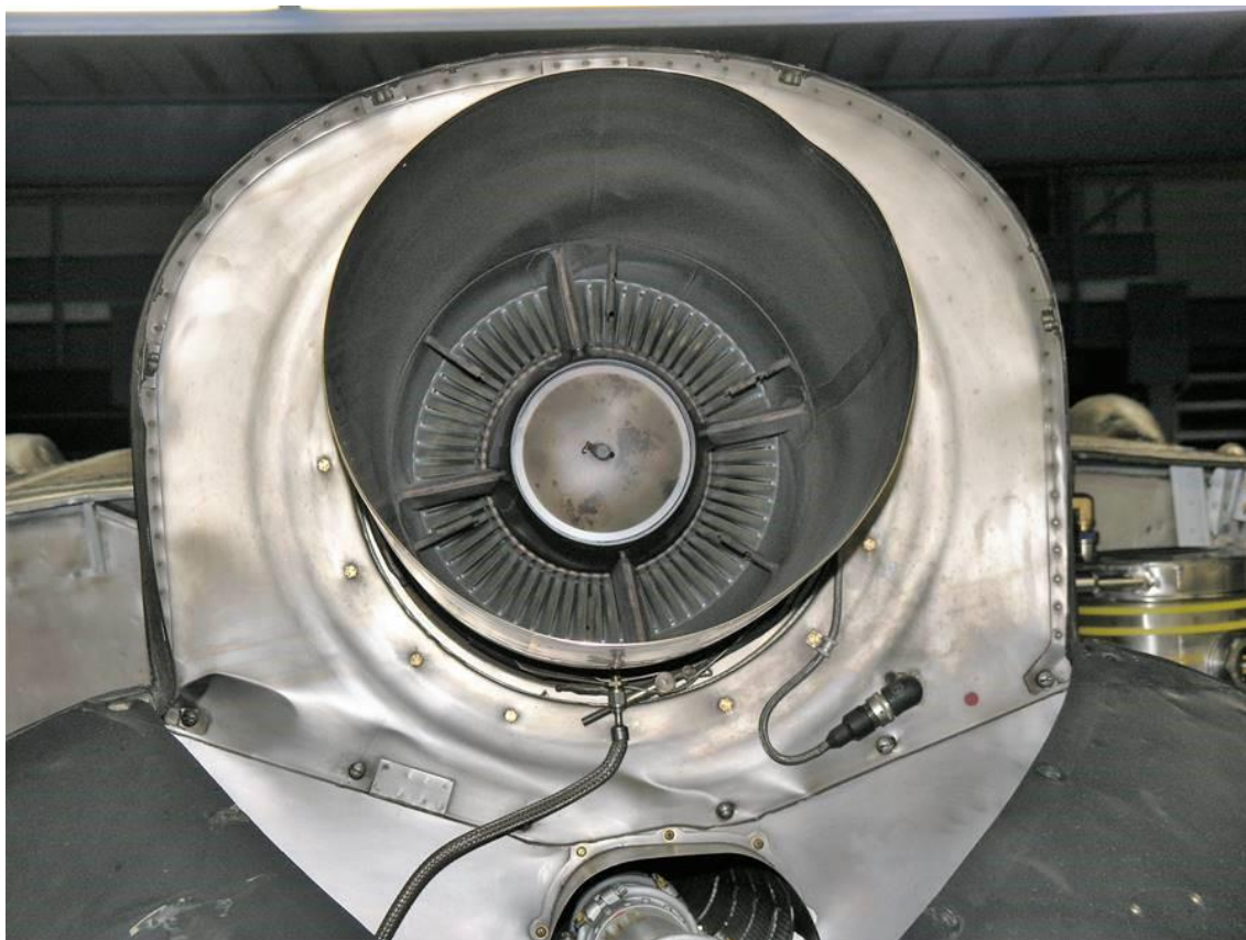
Figure 11: Typical exhaust, showing accessibility for inspection
