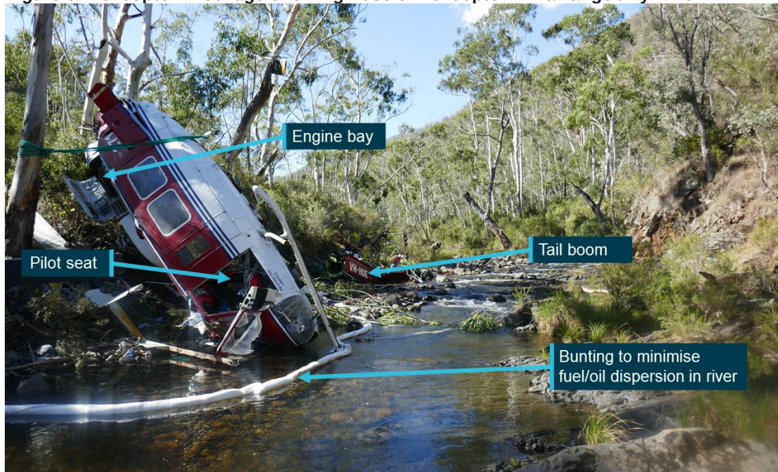
Figure 5: Helicopter wreckage showing nose of helicopter in Yarrangobilly River
