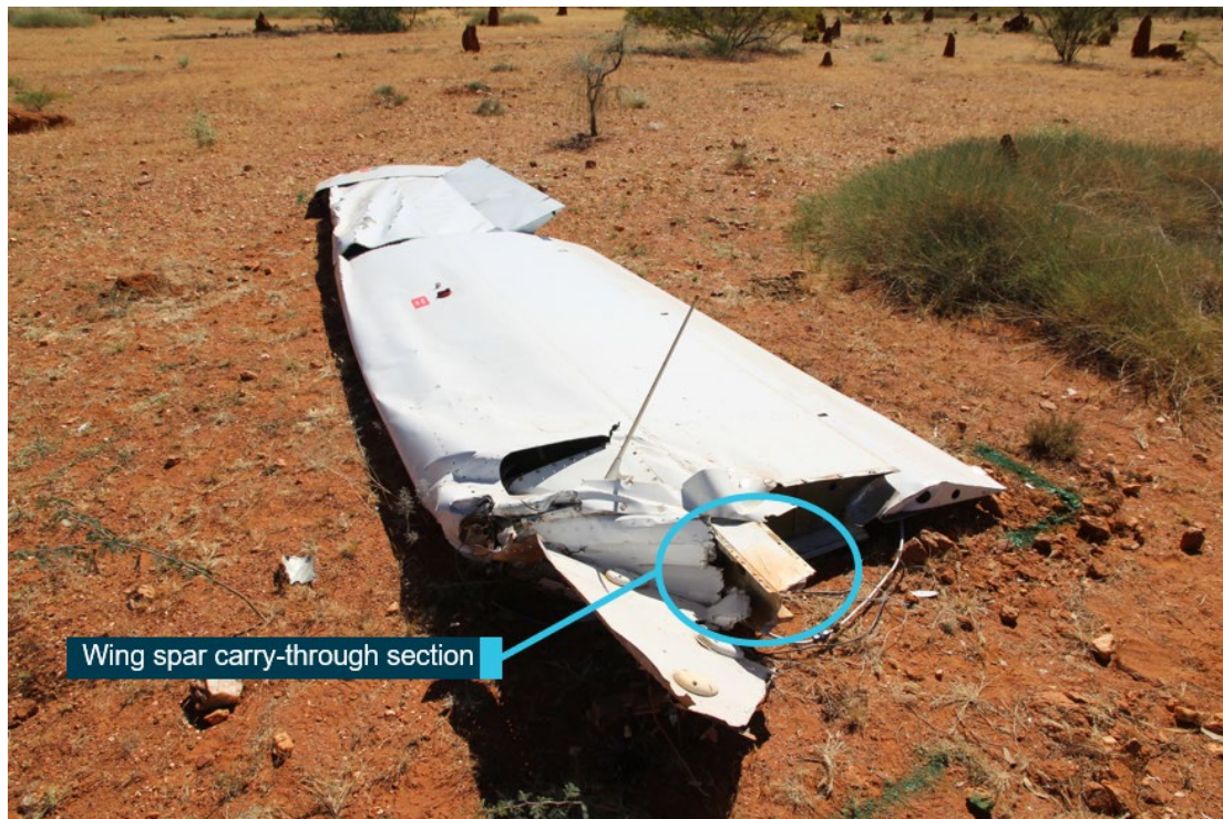
Figure 11: Separated right wing viewed from the inboard end
