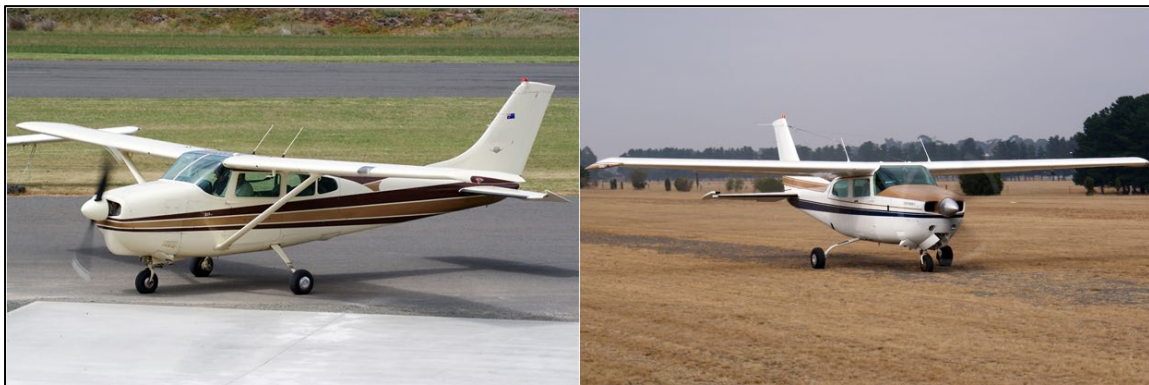
Figure 3: A 1960 C210A with wing struts (left) and a 1980, cantilever winged, C210N (right)
