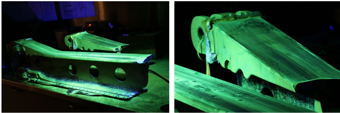
Figure 23: Composite image of the carry-through spar during liquid fluorescent penetrant inspection
