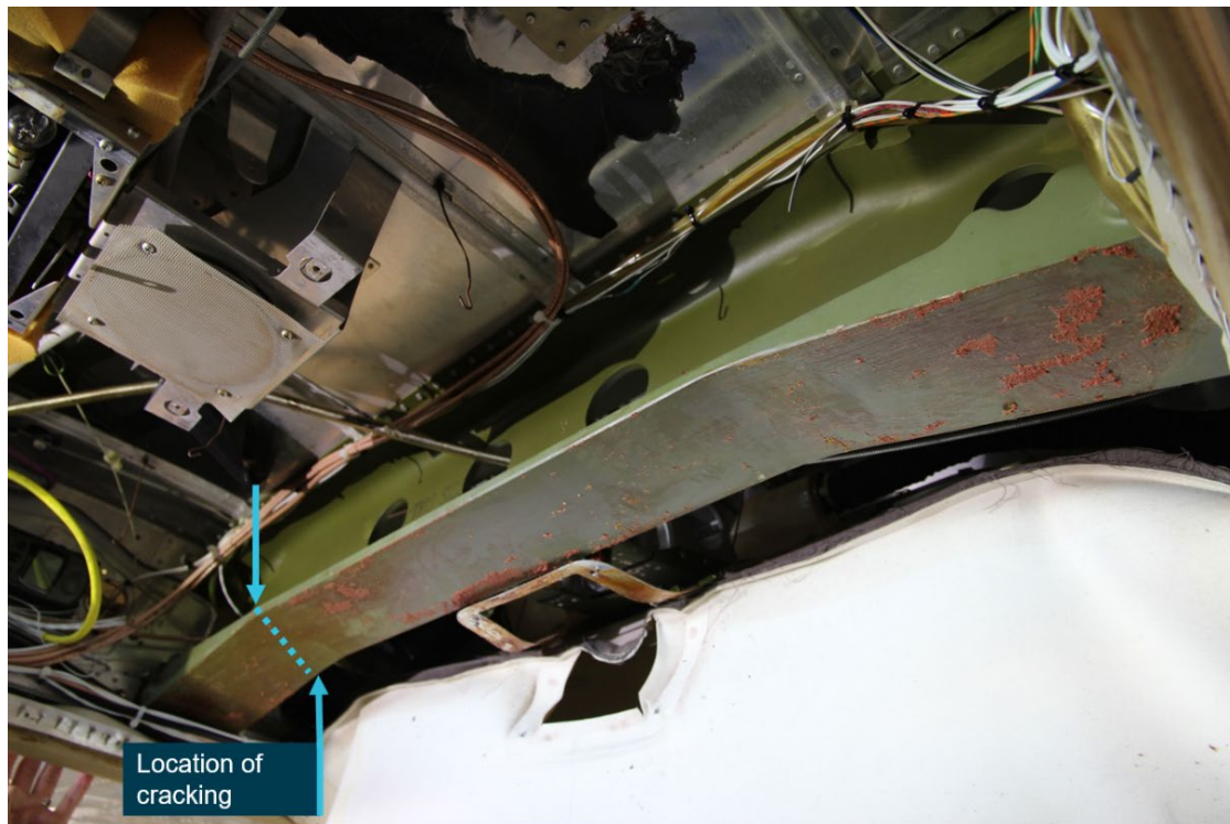
Figure 14: An exemplar Cessna 210N wing spar showing the approximate location where cracking had developed on the carry-through from SUX
