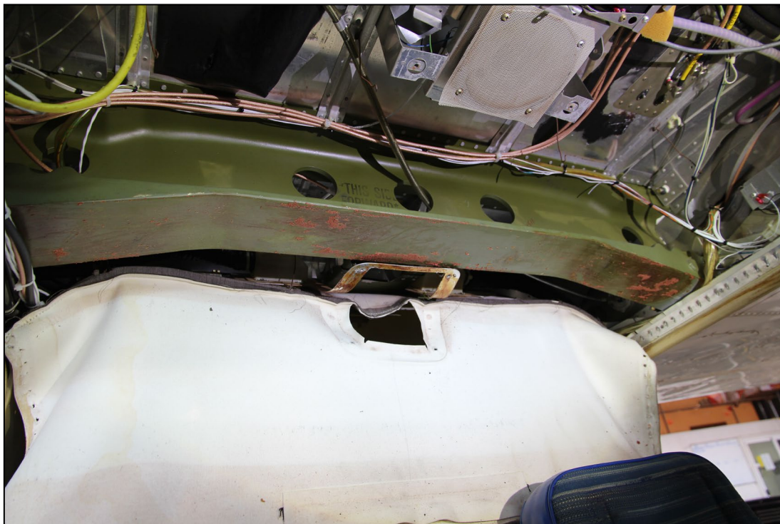
Figure 23: View of the carry-through structure looking aft with the cabin lining removed
