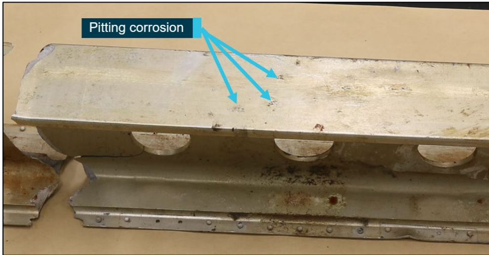
Figure 16: Carry-through underside surface showing pitting corrosion.
