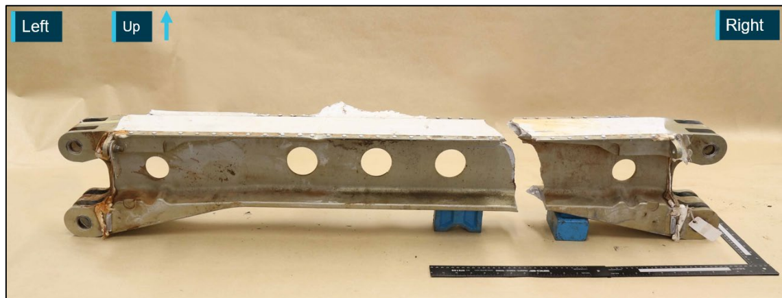
Figure 15: The carry-through spar in the ATSB laboratory
