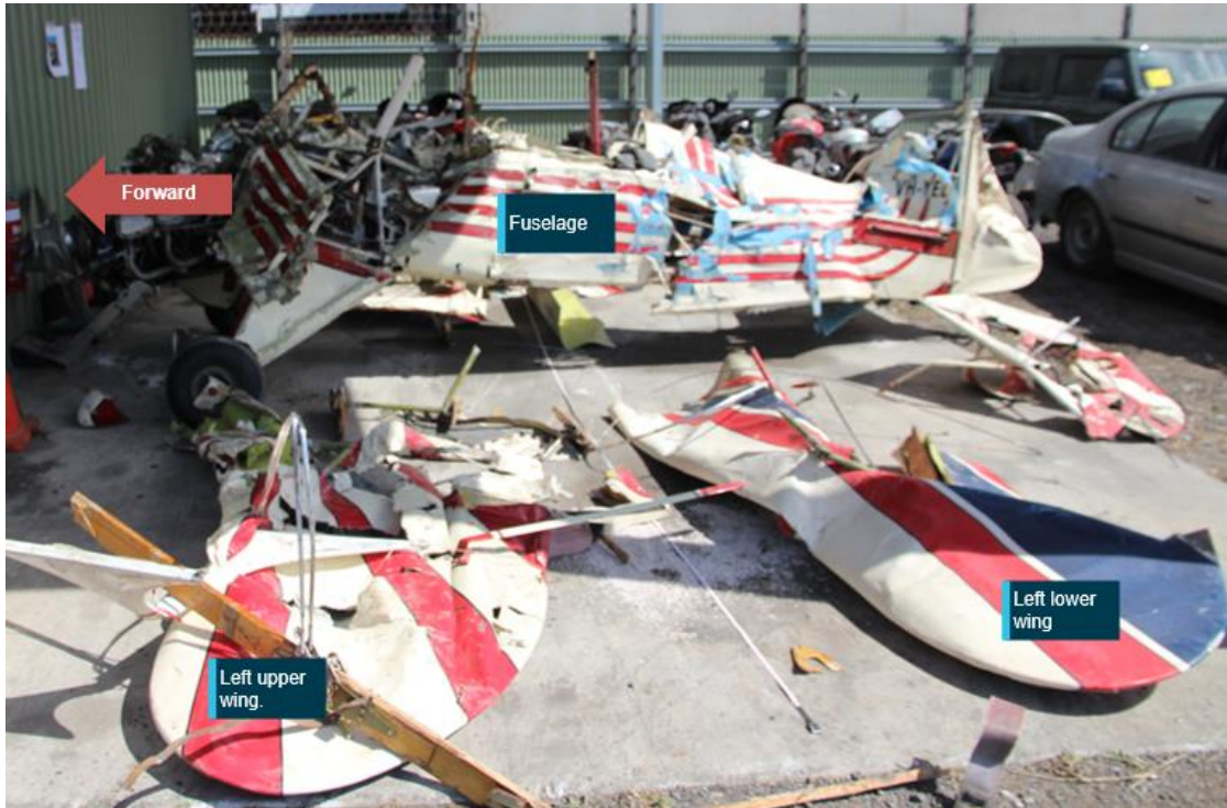
Figure 6: VH-YEL as recovered and partially reassembled
