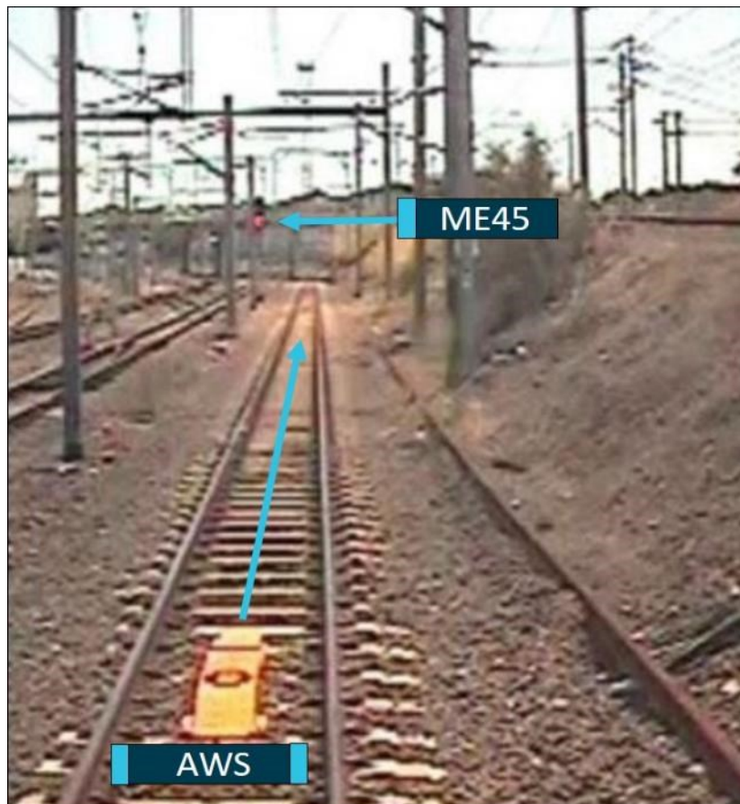
Figure 6: Automatic warning system (AWS) magnet and signal ME45 displaying a red (stop) aspect
