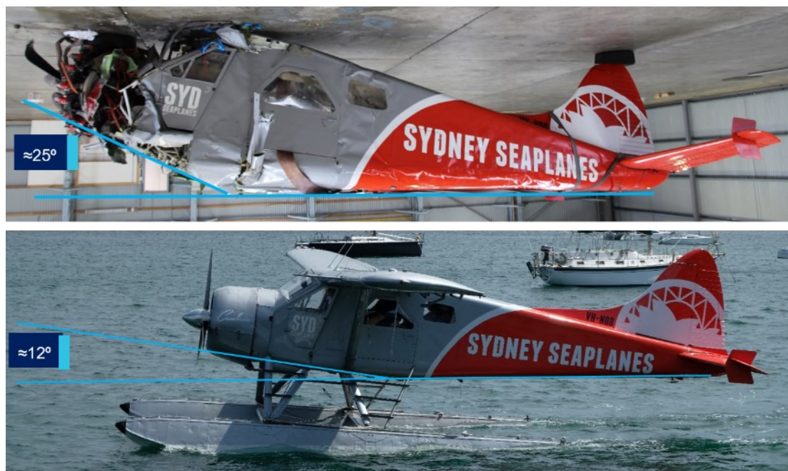
Figure 2: Engine and forward fuselage deformation post-accident (top) with pre-accident nose to rear fuselage angle (bottom)
