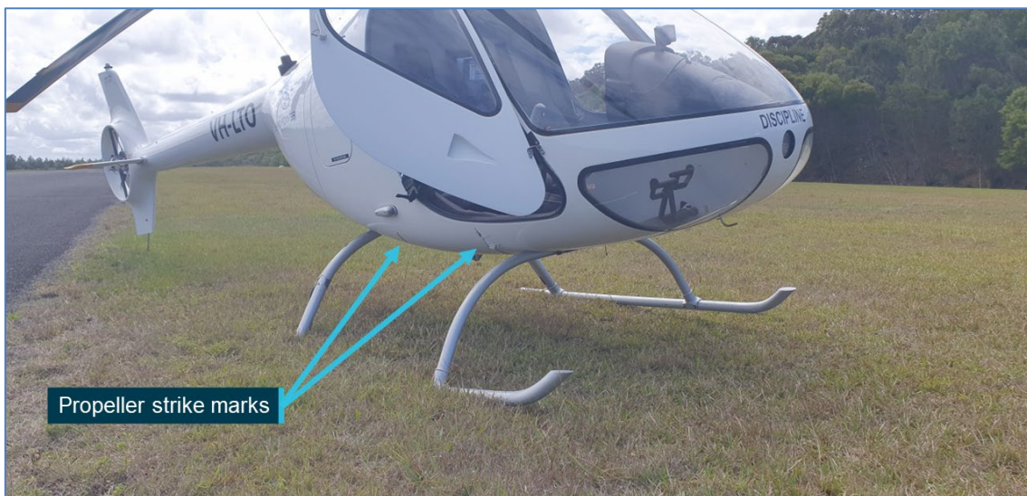
Figure 1: Propeller strike mark and skid damage to VH-LTO
