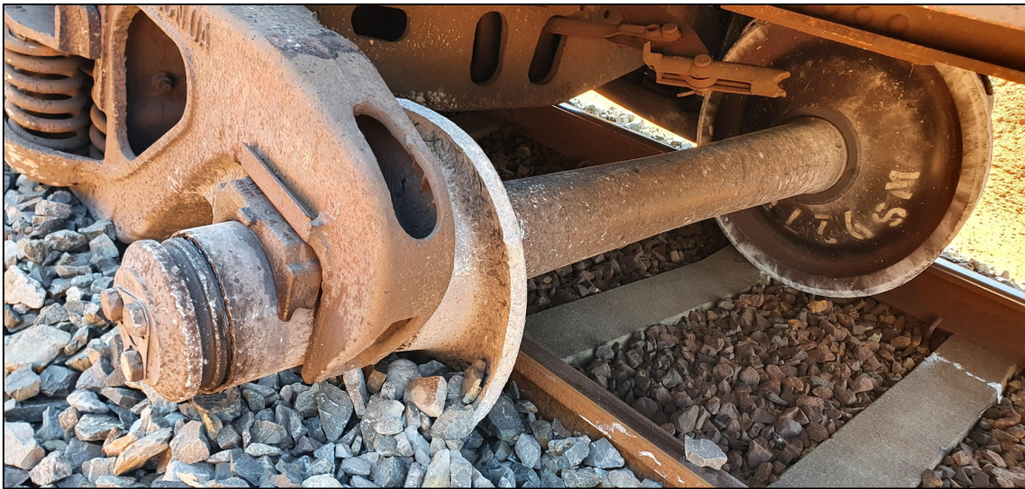
Figure 1: The derailed wheelset on ARFY2253s
