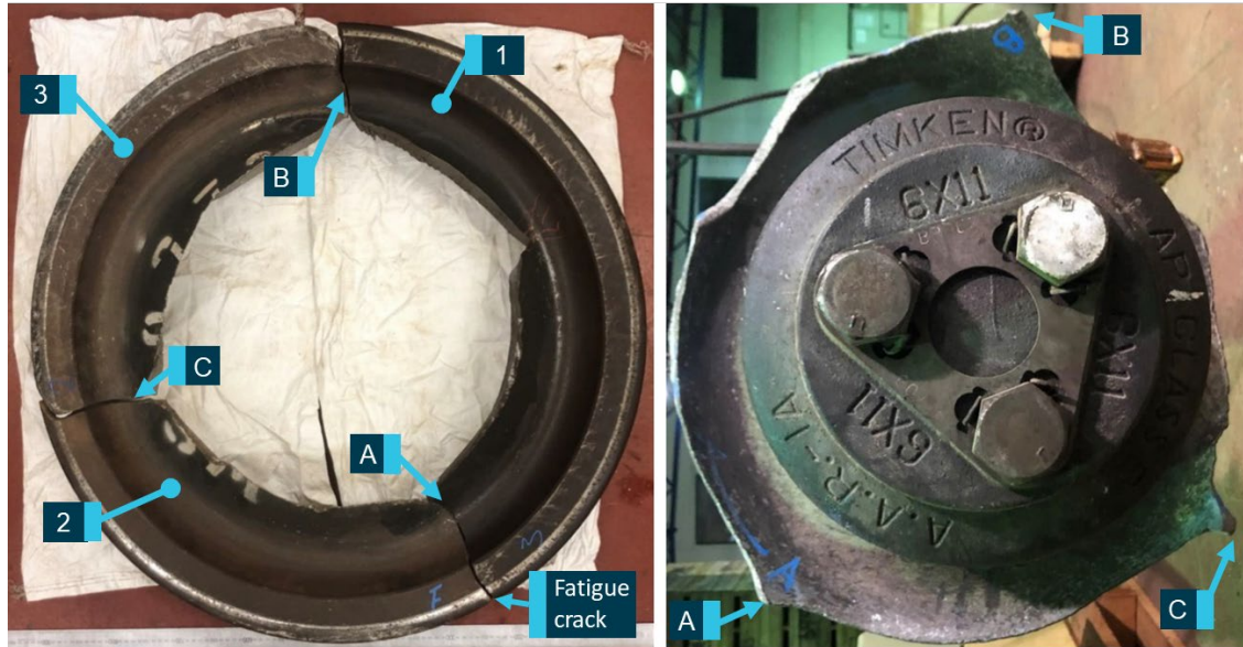
Figure 2: Reassembled wheel fragments (left) and wheel hub (right)
