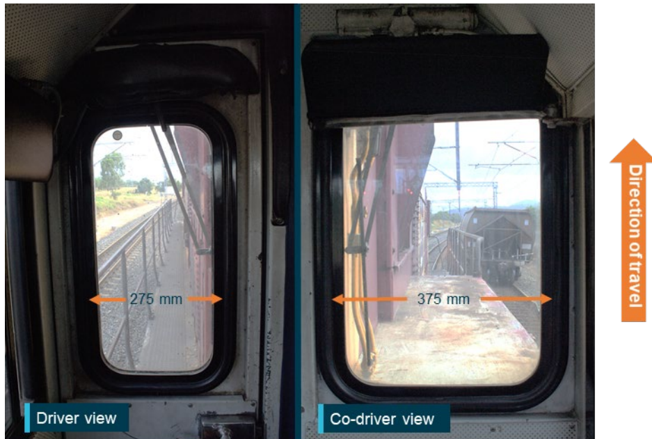
Figure 8: View from inside the cabin from driver and co-driver perspective with long end leading
