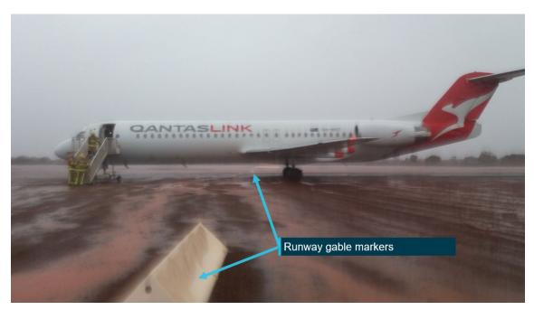
Figure 2: Image taken of the aircraft stopped within the runway end safety area
