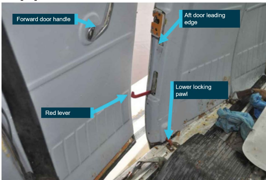
Figure 7: Cessna 206 forward cargo door open showing red lever activated on the leading edge of rear door
