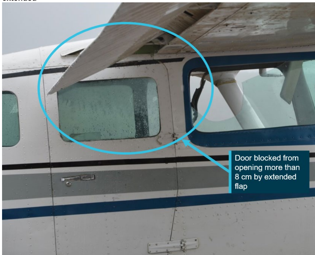
Figure 6: Cessna U206 with door unable to be opened more than 8 cm when flap is extended
