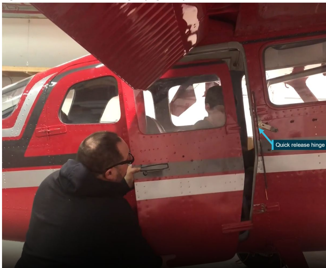
Figure 10: Cessna U206 with emergency egress system
