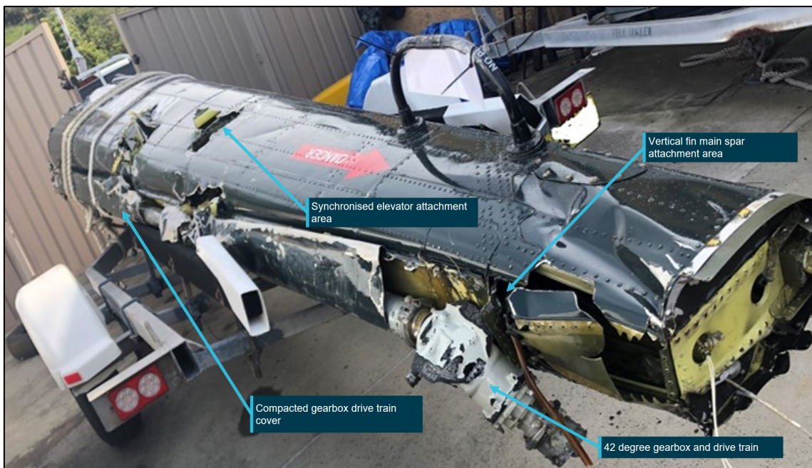
Figure 8: VH-UVC tailboom following recovery from the ocean floor
