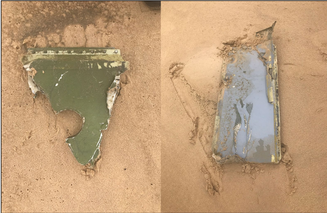
Figure 7: Items of honeycomb construction found on Stockton Beach, probably from UVC
