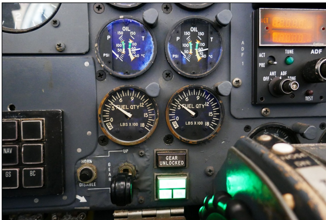
Figure 3: Fuel quantity gauges after defueling in Broome
