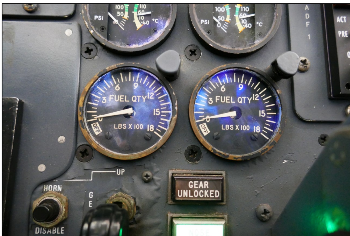
Figure 4: Fuel quantity gauges after cleaning and drying the probes
