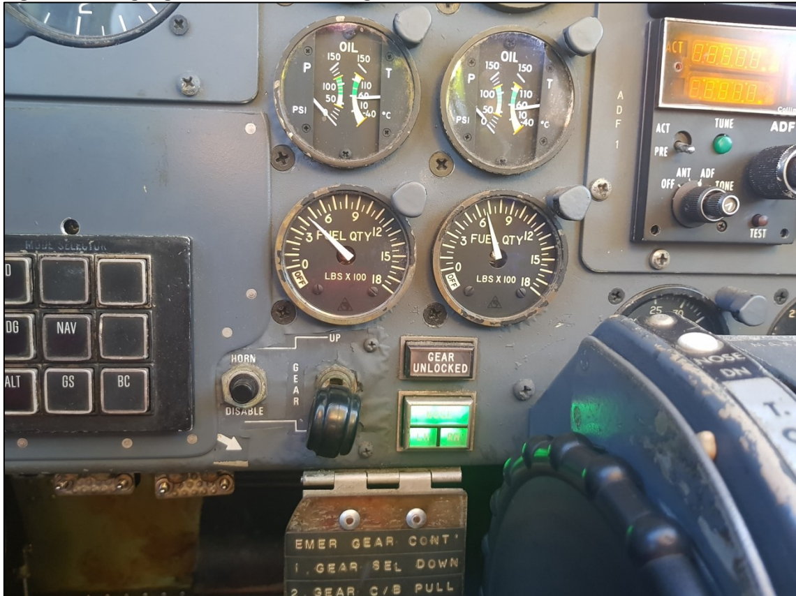
Figure 2: Fuel gauges after forced landing
