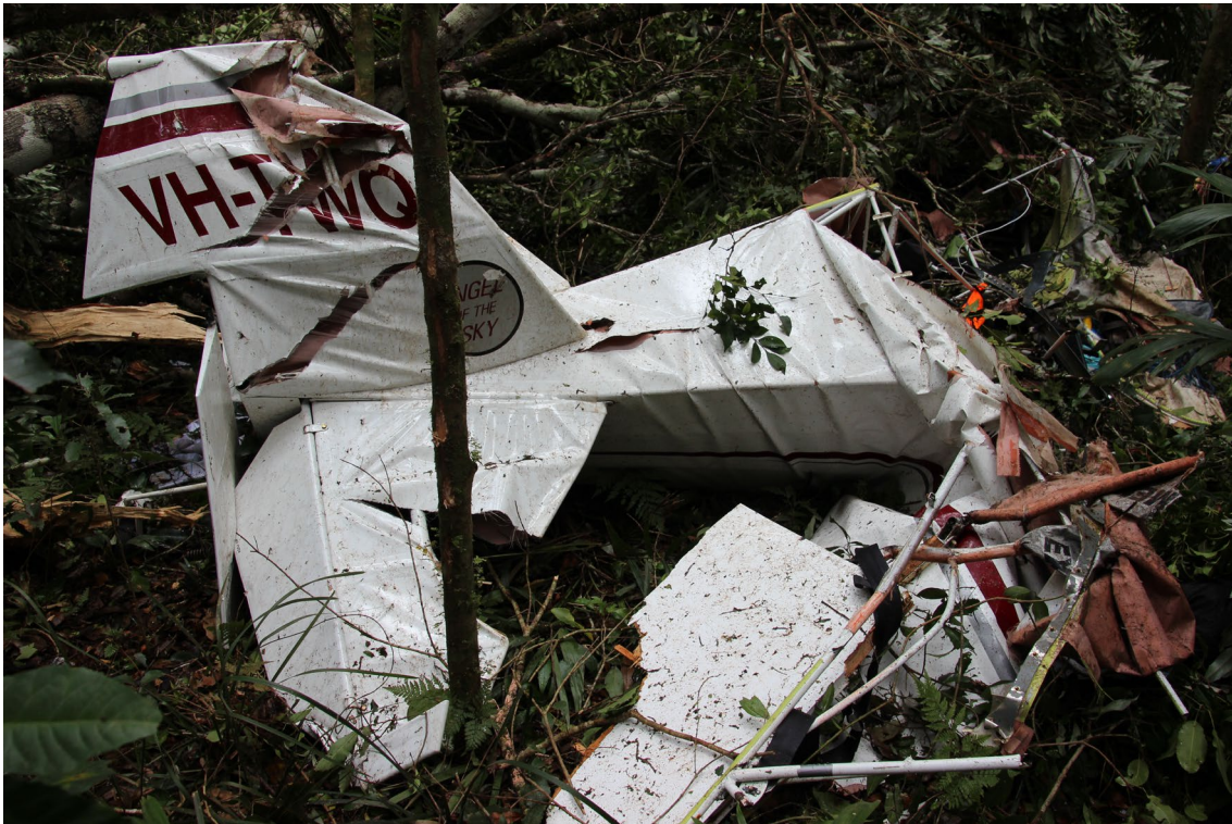
Figure 3 - VH-TWQ's empennage at the accident site
