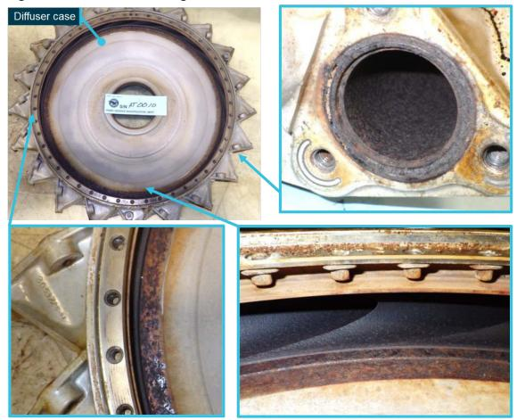
Figure 2: Diffuser case showing areas of corrosion
