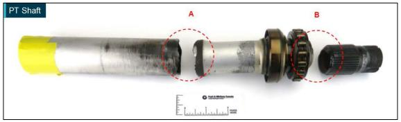
Circled locations A and B refer to the two different fracture surfaces Source: P&WC
