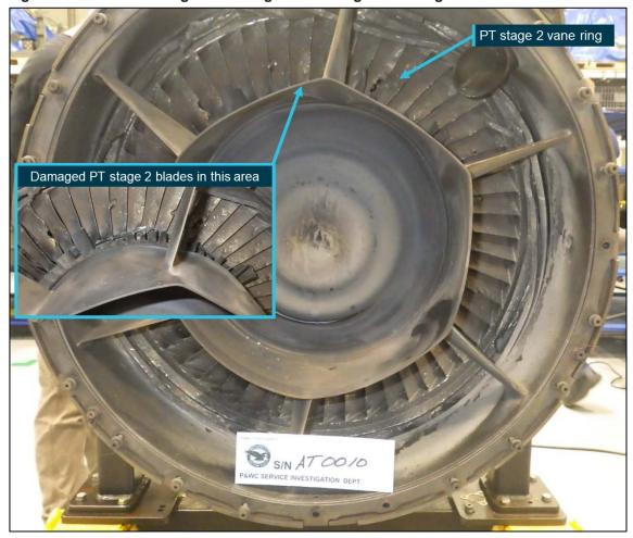
Figure 1: Rear-view of engine showing second-stage PT damage
