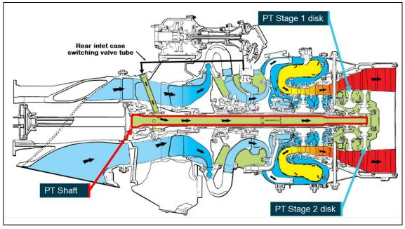
Figure 6: PW100 series air system
