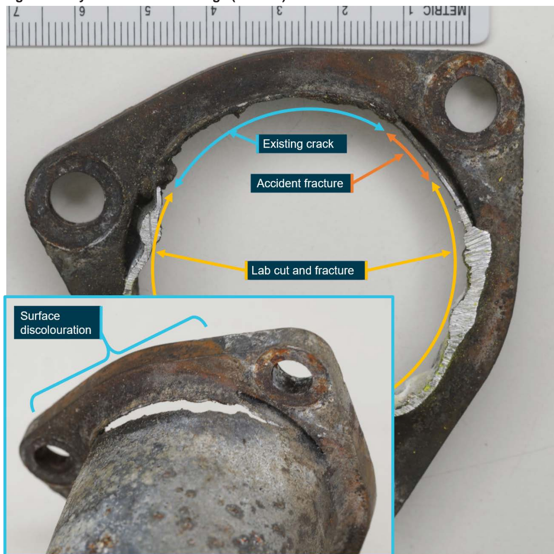
Figure 26: Cylinder 7 exhaust flange (detail E)
