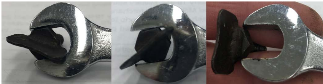
Figure 29: Spanner accessibility on AN3 modified bolt
