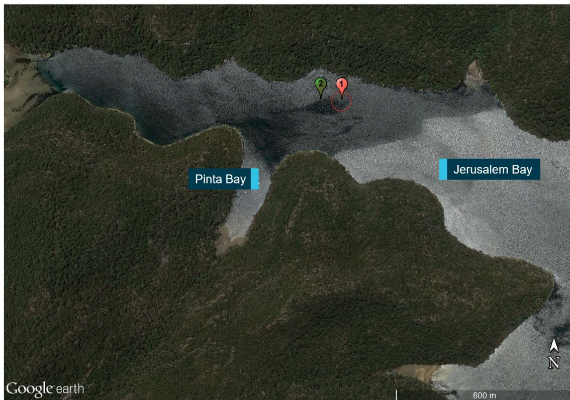
Figure 17: Location of the initial impact (circled) with the windscreen/left wing (1) and fuselage/tail/right wing floats (2) locations on the riverbed
