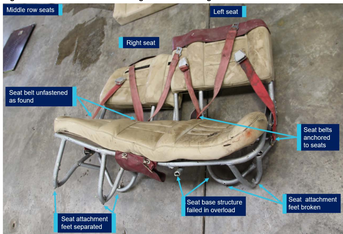
Figure 33: Middle row seats showing structural damage and seatbelts
