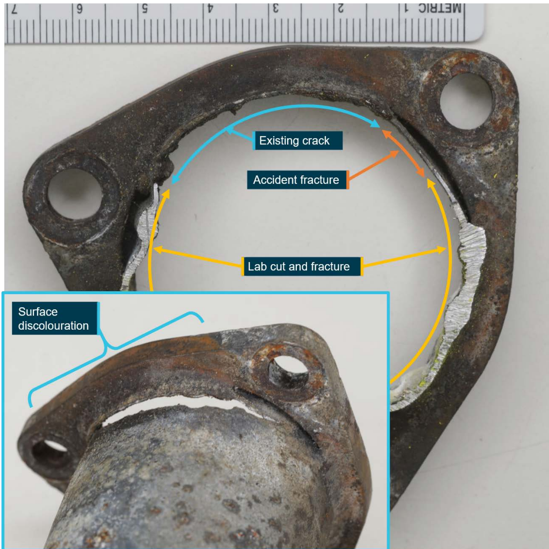
Figure 49: Cylinder number 7 exhaust flange crack (detail E)
