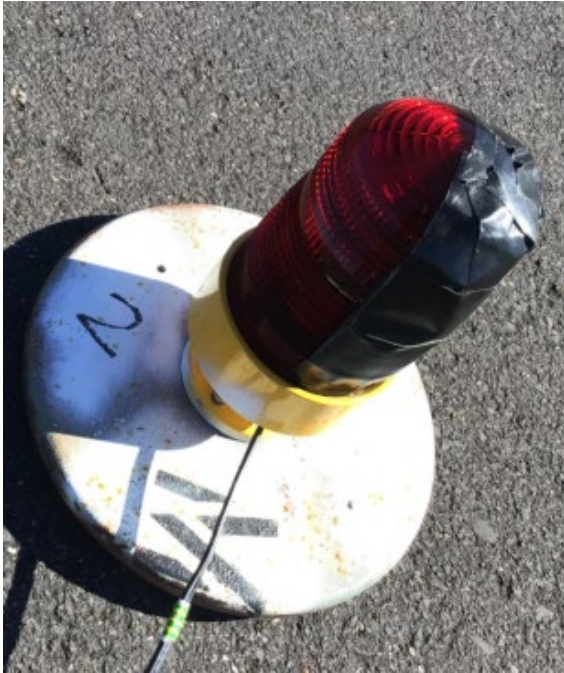
Figure 1: Example of temporary runway end light – taped to be unidirectional
