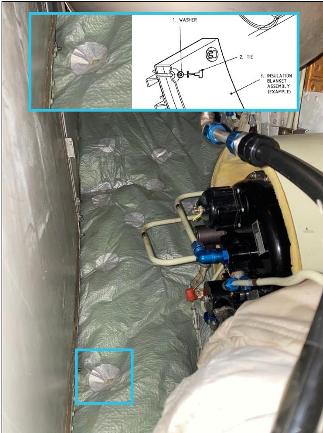
Figure 6: Typical insulation blanket installation using the plastic ties
