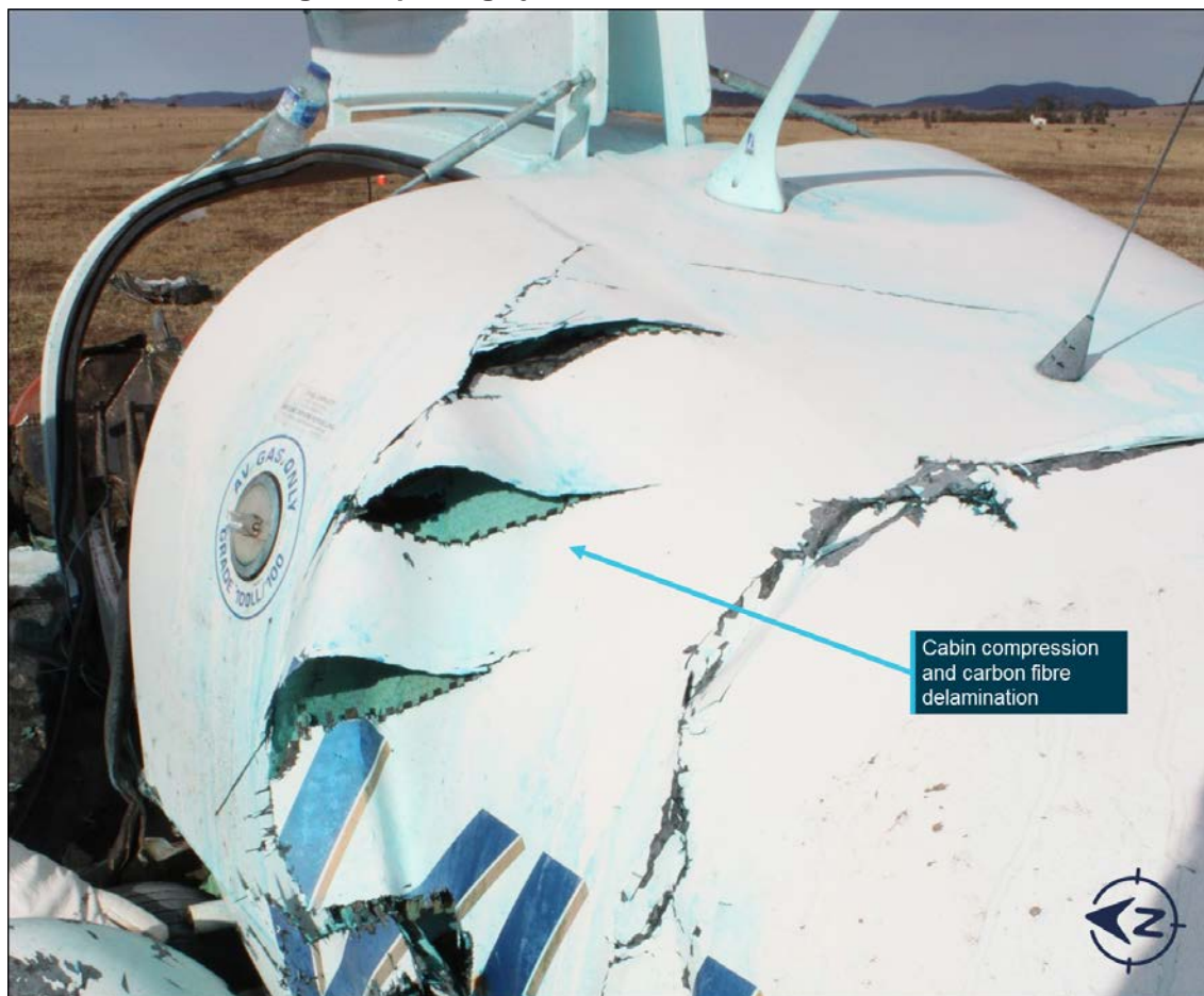
Figure 4: VH-XLK rear fuselage section showing compression damage to composite structure and creasing at empennage junction
