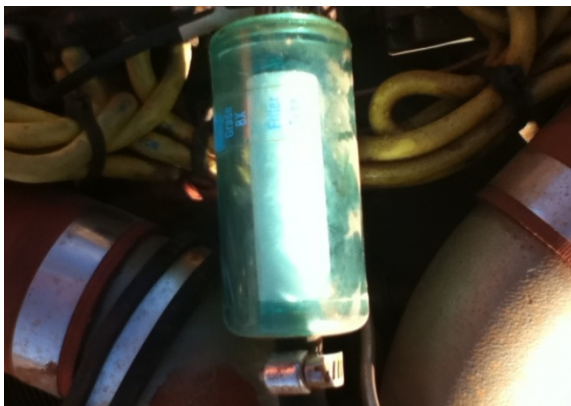
Figure 2: Empty fuel filter in engine bay.
