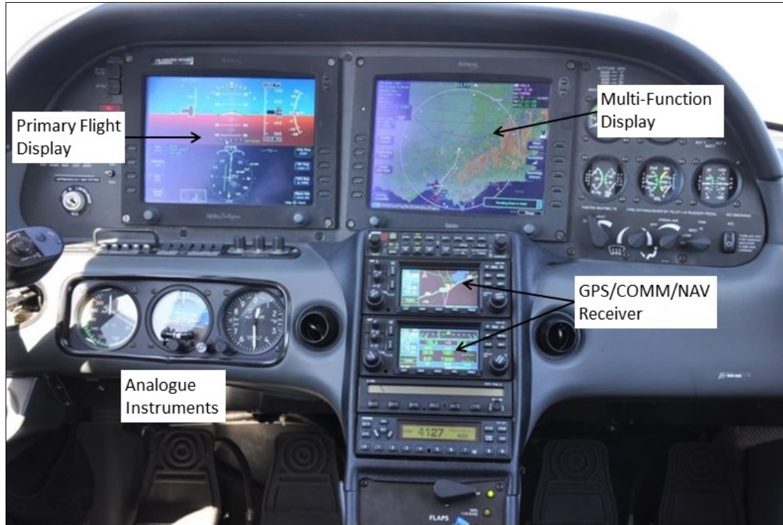
Figure 1: Aircraft instrument panel showing the Primary Flight Display (left screen), the Multi-Function Display (right screen) and analogue instruments during a daylight flight
