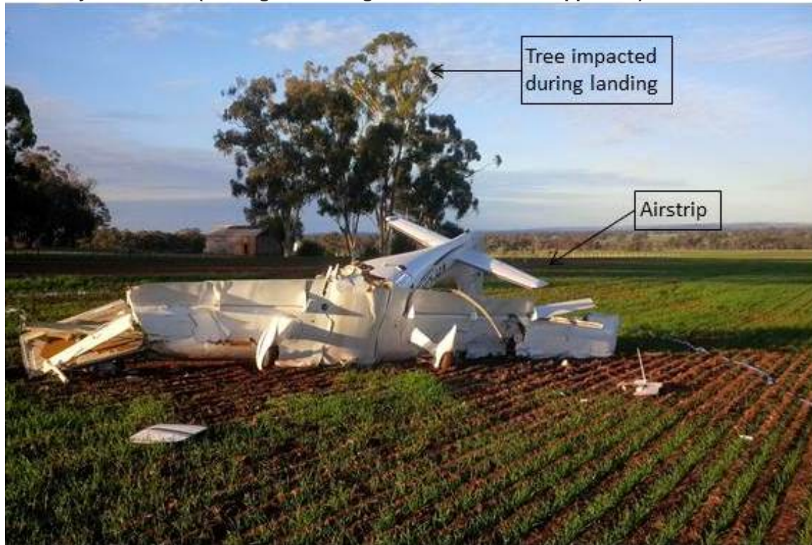
Figure 2: Aircraft wreckage showing the trees adjacent to the airstrip, one of which was struck by the aircraft (looking back along the direction of the approach)
