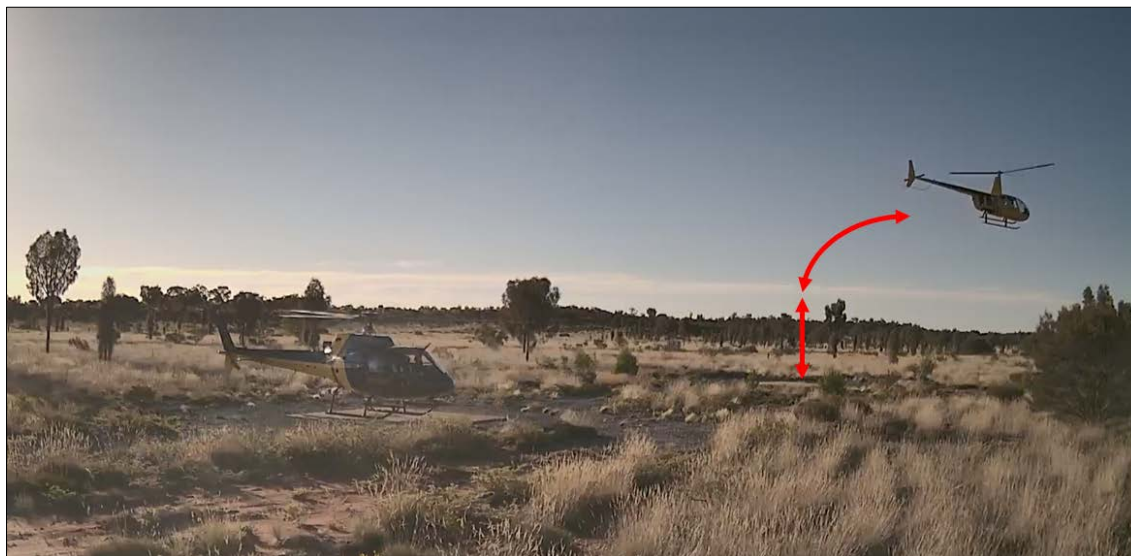
Figure 10: Approximate position of the low rotor RPM warning
