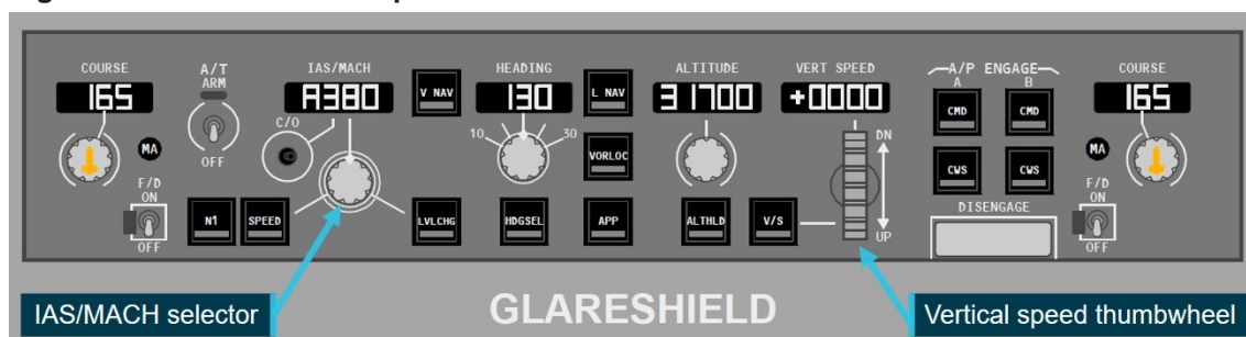
Figure 3: 737 mode control panel
