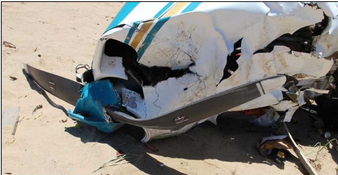
Figure 14: Propeller blades showing slight paint abrasion damage
