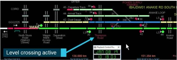
Note: The level crossing fault alarm is a pop-up dialog box, not shown in this image. Time is Central Daylight-saving Time (CDT), Coordinated Universal Time (UTC) +10.5 hours.
