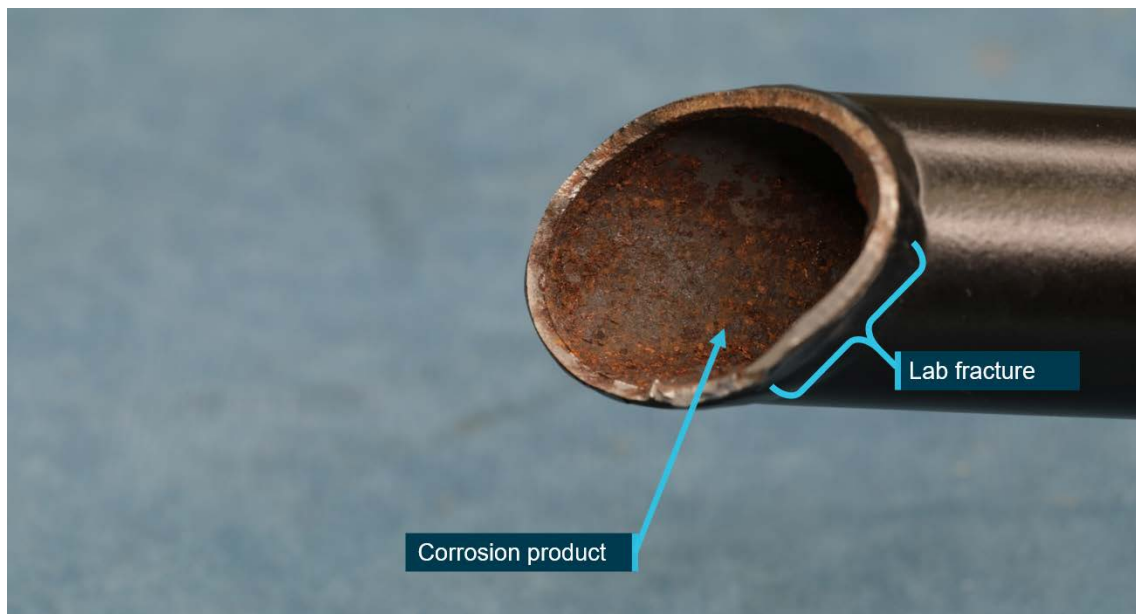
Figure 3: Right tail rotor pedal fracture surface following fracture by the ATSB
