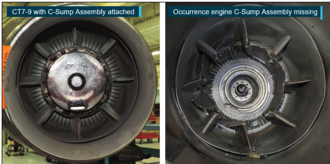
Figure 2: Rear-view comparison of undamaged engine (left) and the occurrence engine missing the C-Sump Assembly (right)
