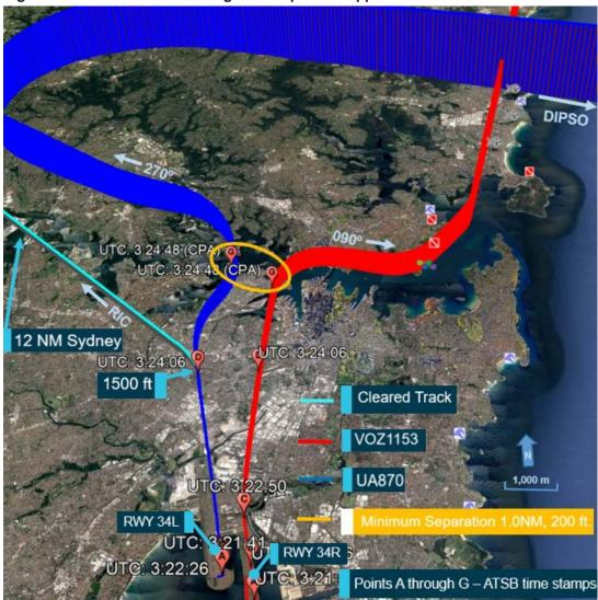
Figure 2: Aircraft tracks showing closest point of approach
