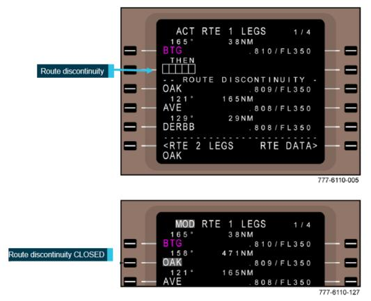
Figure 3: Example of a route discontinuity displayed via the B777 FMC LEGS page
