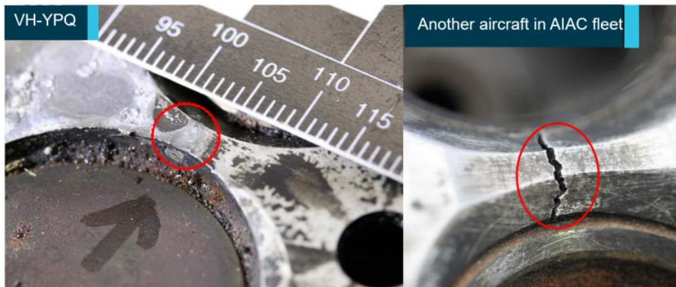
Figure 7: Cylinder cracks in VH-YPQ and another aircraft
