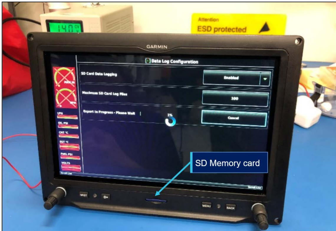
Figure 8: G3X avionics unit being downloaded, showing memory card position
