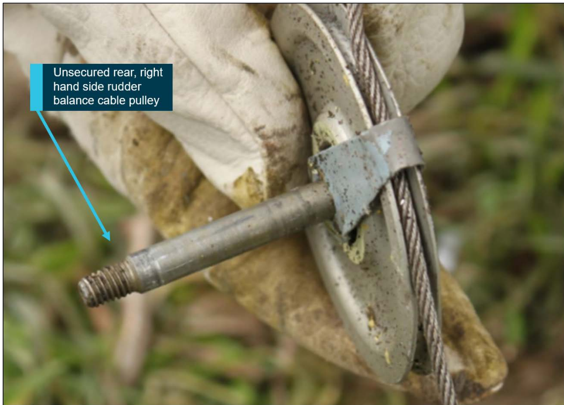
Figure 7: Rear right rudder pulley, found away from the airframe.
