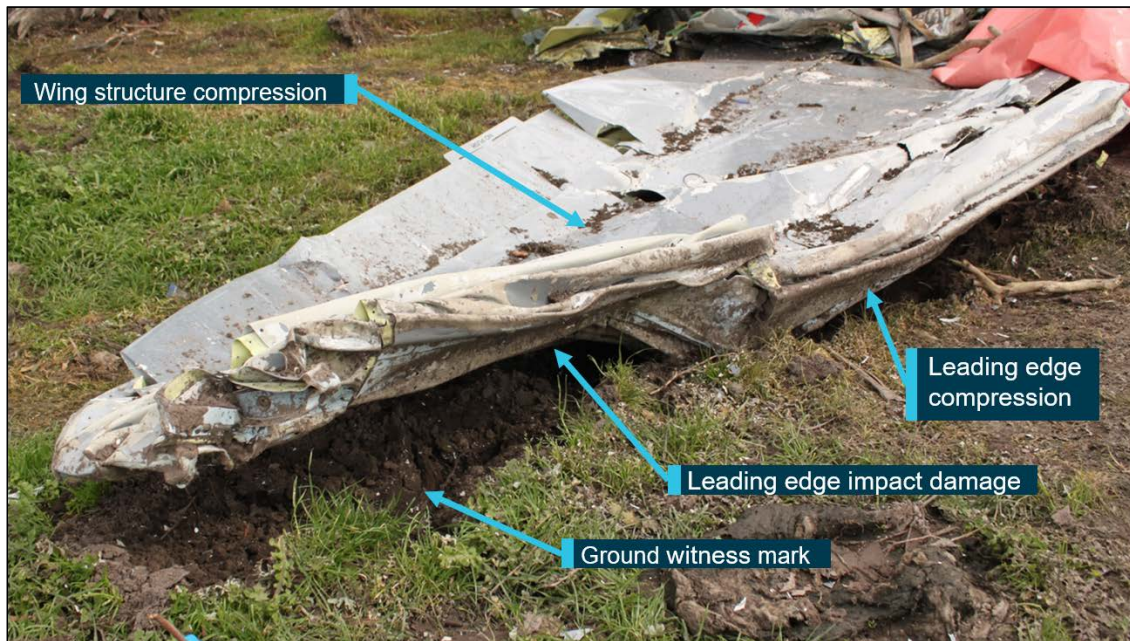
Figure 5: Right wing structure impact damage
