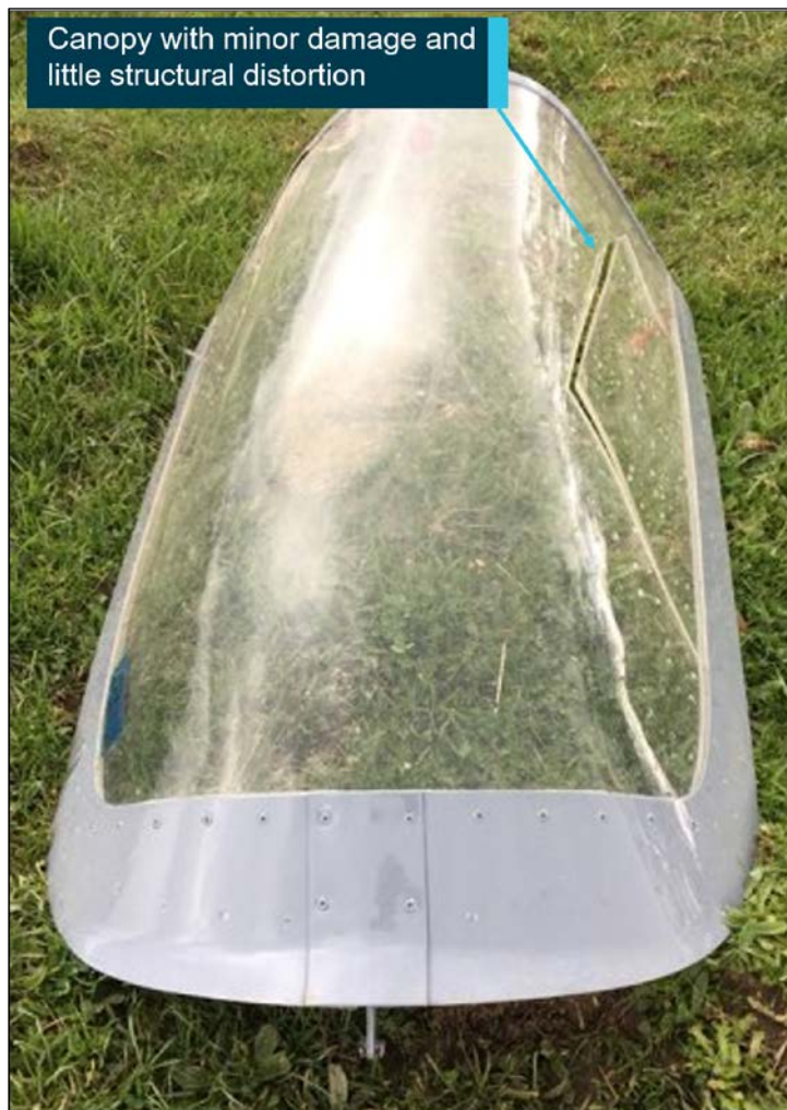
Figure 6: Forward looking view of the rear canopy
