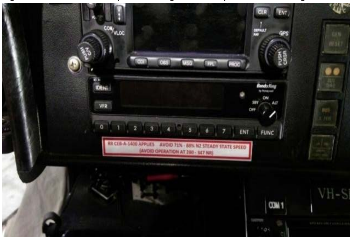
Figure 3: VH-SEV instrument panel showing decal with speed avoidance range
