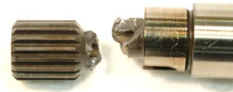
Figure 7: Fractured oil pressure pump shaft
