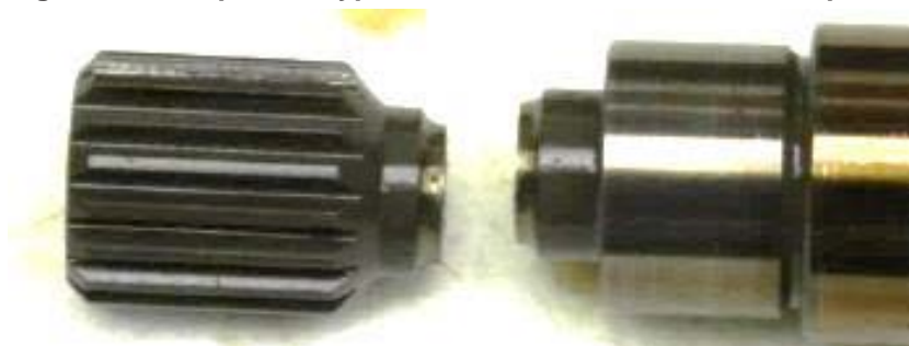
Figure 8: Example of a typical shear neck fracture of an oil pressure pump shaft
