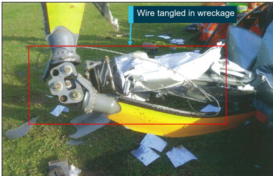
Figure 3: Accident site showing wire tangled in the wreckage
