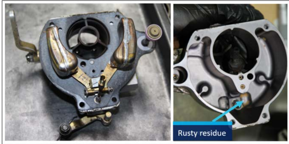
Figure 13: Disassembled carburettor showing internal components
