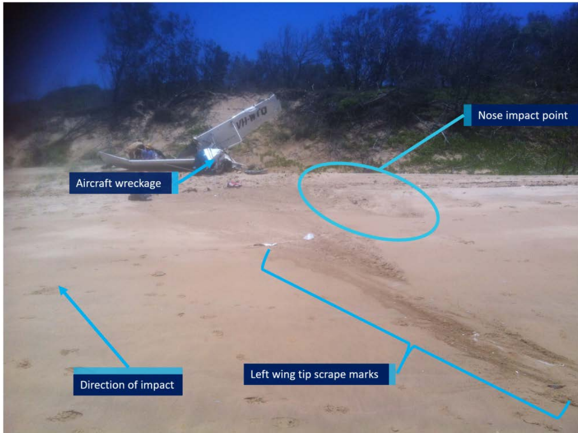
Figure 8: VH-WTQ accident site showing impact marks
