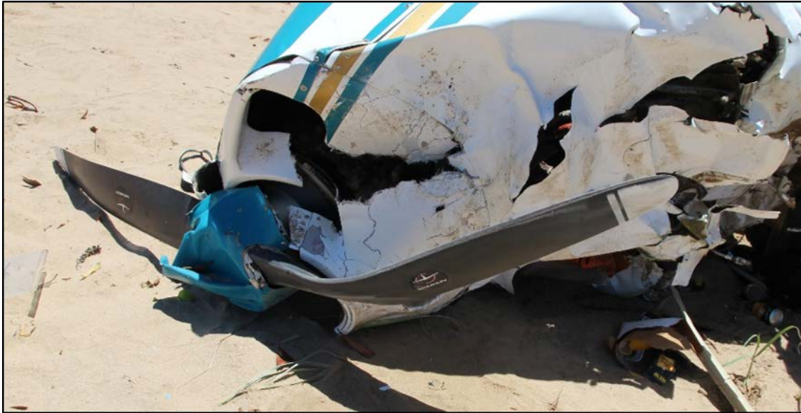
Figure 14: Propeller blades showing slight paint abrasion damage
